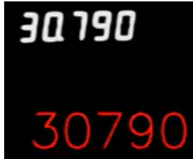
(a) Example frame of OCR score recognition from camera. Actual score in white, detected in red.
