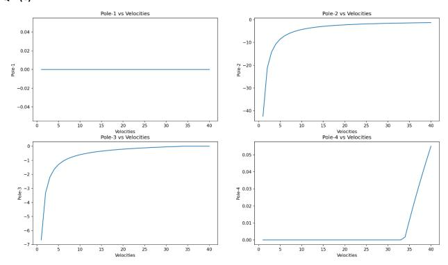
Apart from Pole-1 (which is constant at the origin), the other poles increase in value and go towards zero. Hence, the stability of the system decreases with increasing velocity.
