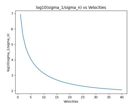
Since the ratio of sigma\_1 and sigma\_n is decreasing with increasing velocity, it implies that the singular value corresponding to the least controllable state is increasing. Hence, the controllability increases.
